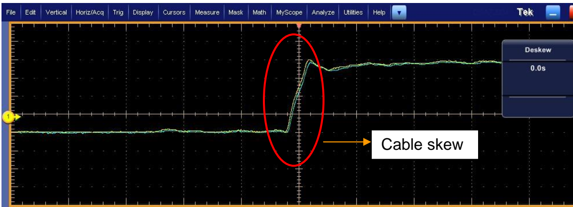
Figure 5: Visible Cable Skew
