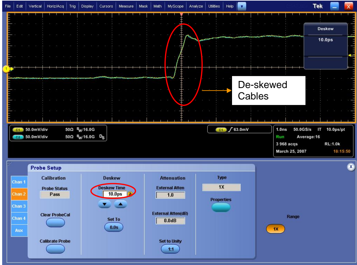
Figure 6: Cable Skew Adjusted
